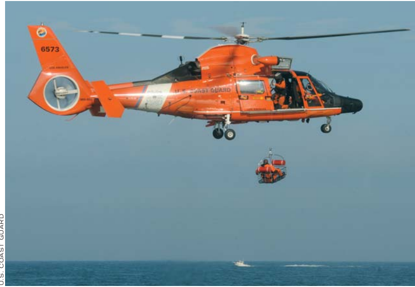
U.S. COAST GUARD An MH-65C Dolphin helicopter aircrew from Air Station Los Angeles hoists a flight mechanic during annual wet drills Sept. 15 off Redondo Beach, Calif.
